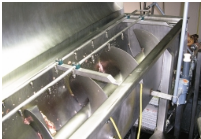
At Jensen Meat, an antimicrobial is sprayed on ground beef as the meat is screw-conveyed to a grinder. (Photo courtesy Jensen Meat.)
